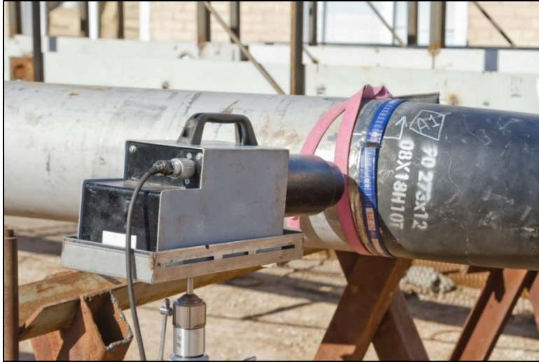
Fig.no.6.4- A setup showing a radiography camera in operation near a large pipeline structure
